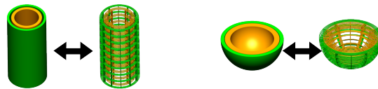
Figure 1: Examples of two benchmarking data sets: inflation of cylindrical and spherical thick-walled shells, visualised with cmGUI ( www.cmiss.org/cmgui ).
